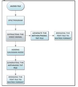
Flowchart depicting the conversion of voice signal to text files i.e. with noise and without noise.
